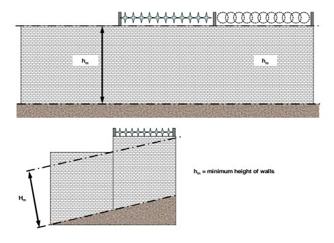
Figure 2 Minimum height of free-standing barriers - mesh and panel fencing
