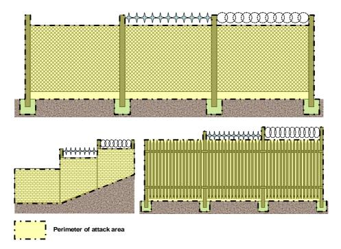
Note: Toppings that are not tested and rated as part of the free-standing barrier may not offer resistance to penetration equivalent to that achieved by the free-standing barrier and may even undermine the security rating achieved by the free-standing barrier. Care should therefore be taken to ensure the compatibility of toppings and the fixing methods to be employed and to ensure that their use does not invalidate any security rating attributed to the free-standing barrier.
